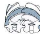
Fig 2 As the rotors mesh, the gas is trapped between the rotors and the casing.
